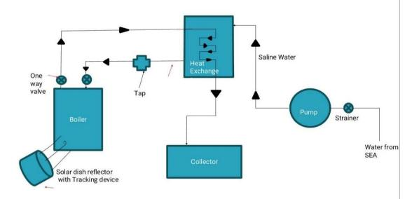
Desalination process can be implemented using following steps;
