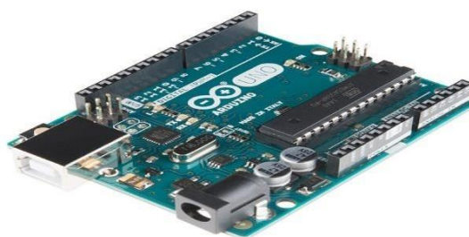
FIG II. Arduino uno development board
