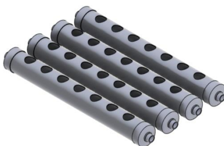
Fig 4.3: An example of vertical stacking of PVC pipes for Hydroponic farming.
