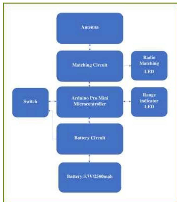
Figure. 2: Flowchart for RF Energy Harvesting
