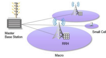
Fig.: C-RAN architecture
