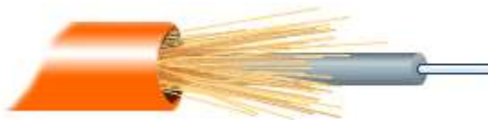
Fig.8 Fiber optic cable
