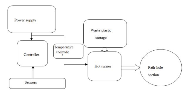
Fig 3.1: Block Diagram of Implementation Technology to Repair Pothole Using Waste Plastic
