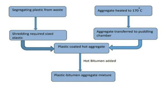
Fig. 3.2 Process of aggregate mixing
