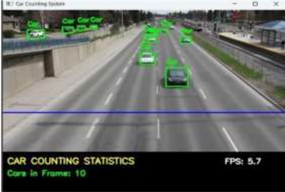
Fig. 2. Vehicle detection using YOLO algorithm
