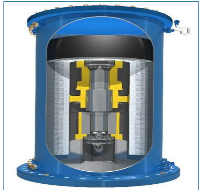
Fig.2 Elements of Flywheels
