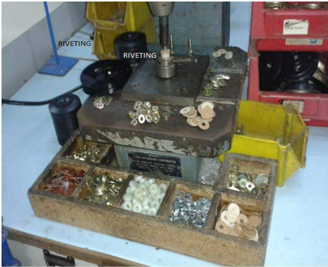
Fig. Old Existed Setup Of Assembling Of Horn Diaphragm
