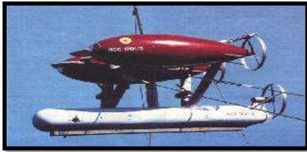
Figure 1.1 Autonomous Benthic Explorer (ABE), Woods Hole Oceanographic Institution (WHOI)
