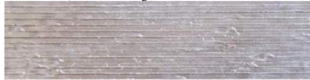
Fig. 5: Surface texture for rough surface (cutting speed 47.1 rpm, depth of cut 0.3 mm, feed 0.4 mm/rev)
